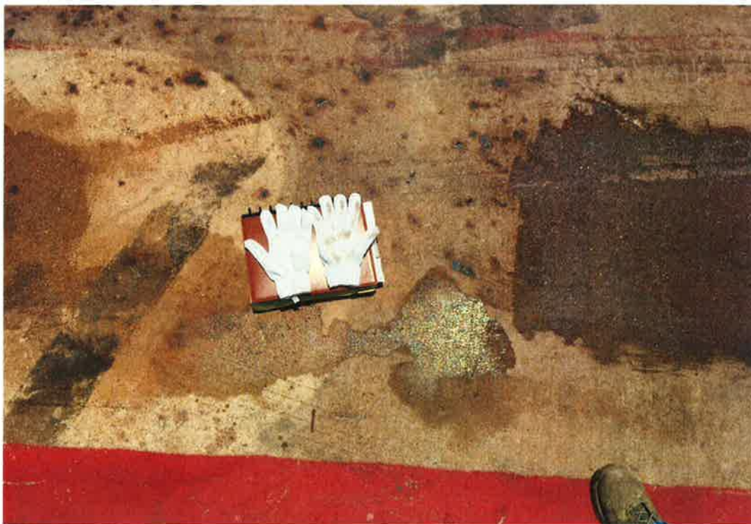
Figure 6. Cleaned Pavement Using HHRU Technology (Left Glove) and Granular Absorbent (Right Glove).
