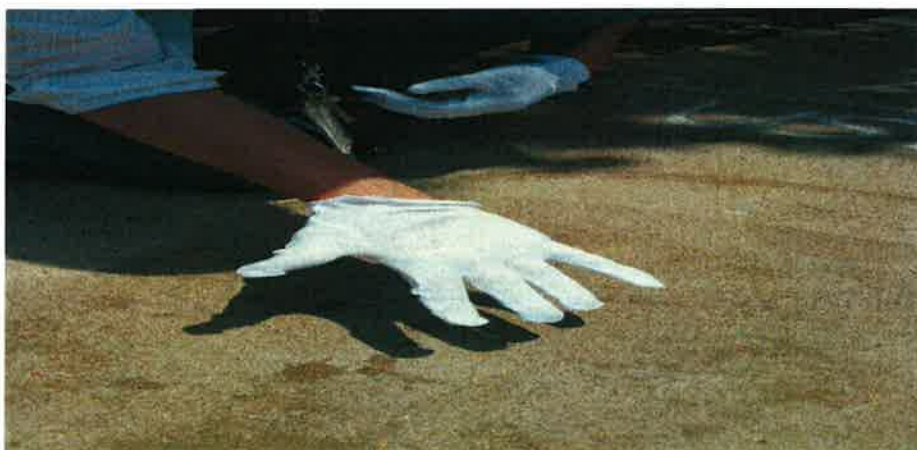
Figure 8. HHRU Glove Test – Residual Oil Visible in Picture
